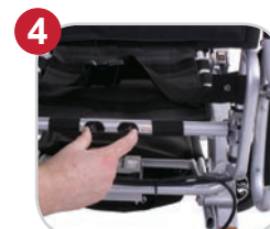
4 Pull the 2 black toggles together (located on the back)
