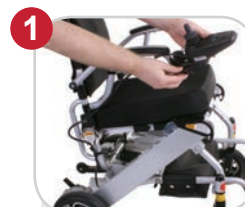
1 Switch off and remove joystick
